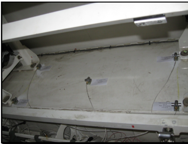
Figure 4. Transducer placement (input to missile rack).
