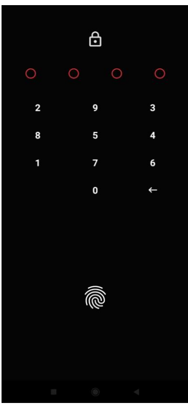
If the « Random Keyboard » option has been set in the User Settings, the numbers of the key pad are shuffled.
